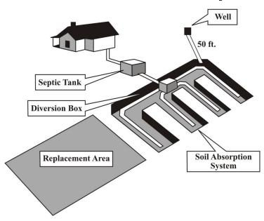
An Onsite Septic System has several components, which consist of a septic tank, a distribution or diversion box (D-box), and a soil absorption field or soil absorption system. Due to the soil composition and the unique features of your property, your system may require an additional dose tank, with a pump and alarm.
